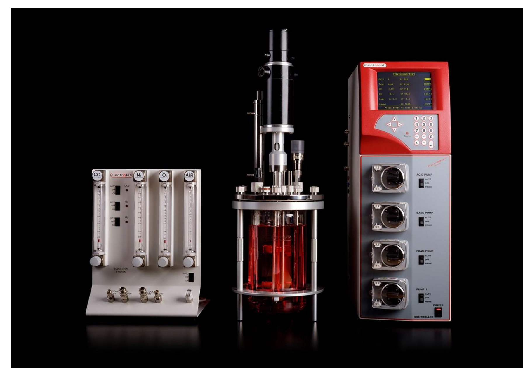
Fig 2. The Electrolab Fermac 320 bioreactor system (Electrolab Biotech, Tewkesbury, England) offers precise control of various environmental factors such as temperature and pH in the process of culturing. (9)
