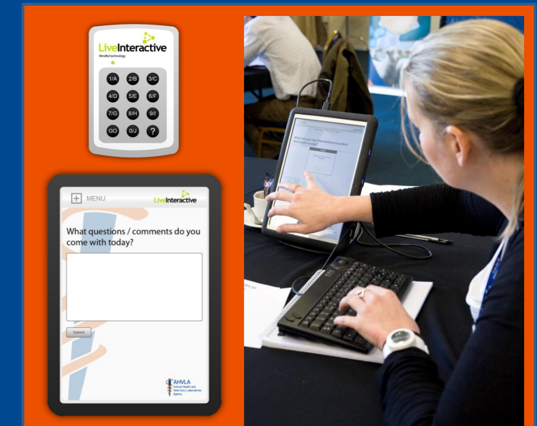
Figure 2 – Individual voting device and delegate messaging tablet, and in action on right.
