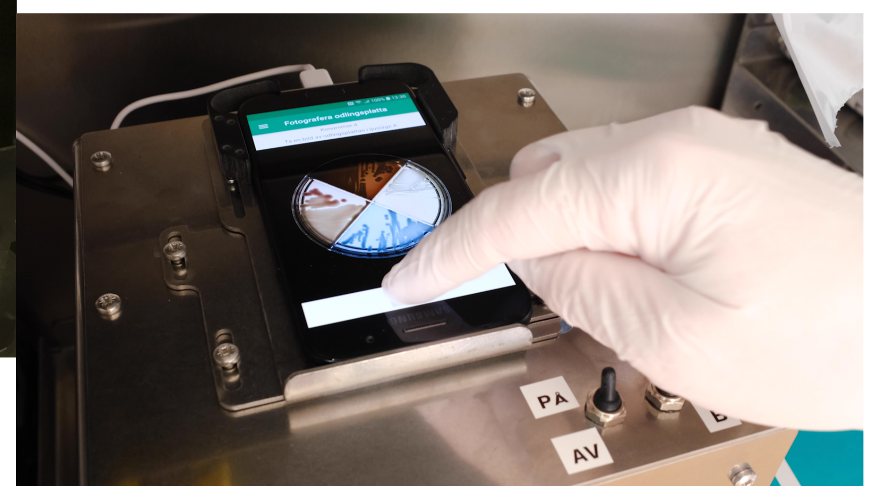
The plate is photographed with a smart-phone camera. After image quality control the growth is classified.
