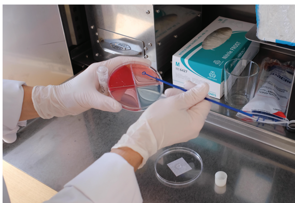
Milk sample collected on the farm is spread on SELMA PLUS agar plates at the farms Bacticam station.
